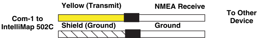
Com-1 wiring to transmit NMEA position information to another NMEA-compatible device.
